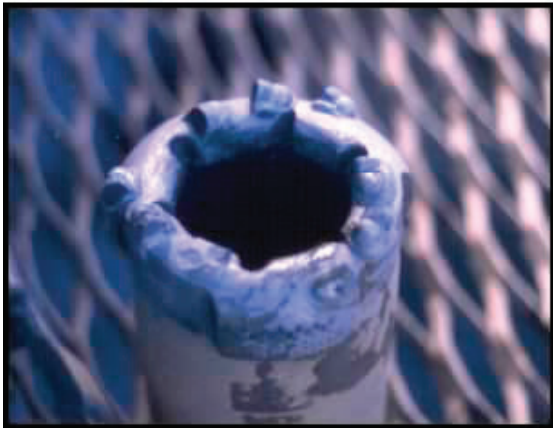
Figure 7.2. Diamond-surfaced core bit for sampling Quaternary sediments.
