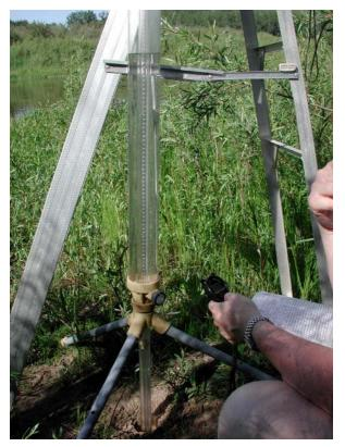
Figure 3.17. Photograph of permeameter testing activities.
