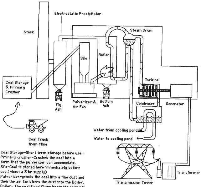
use.(About a 3 hr supply) Pulverizer-grinds the coal into a fine dust and then the air fan blows the dust into the Boiler.
