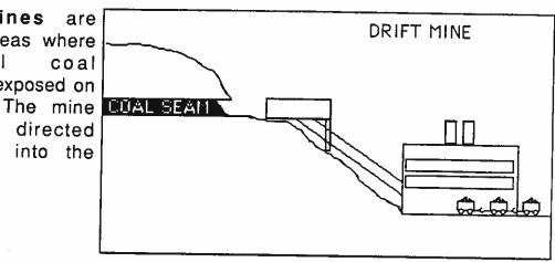
A slope mine involves putting a sloping shaft into the coal seam. The sloping shaft allows a conveyor belt to transport coal, and it allows vehicles to transport men and machines. This method is less expensive than а shaft mine at medium depths.
