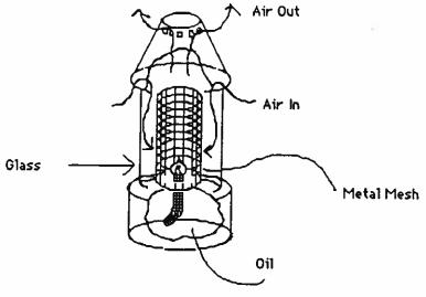
The safety lamp was a major step in advancing mine safety. The flame of this lamp is surrounded bv metal mesh which prevents the flame from igniting Metal Mesh Explosion. The flame will get weak or go in out high concentrations carbon dioxide, and it will burn brighter high concentrations of methane or carbon monoxide.
