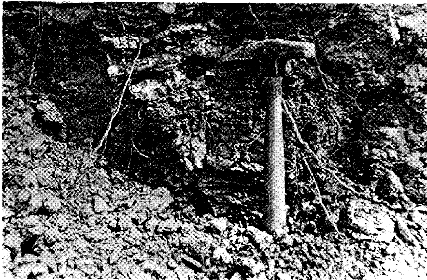
Figure 4—Varved clays; Post-Brown Till lacustrine deposit. Pembina River section; township 52, range 7, west of 5th meridian.
