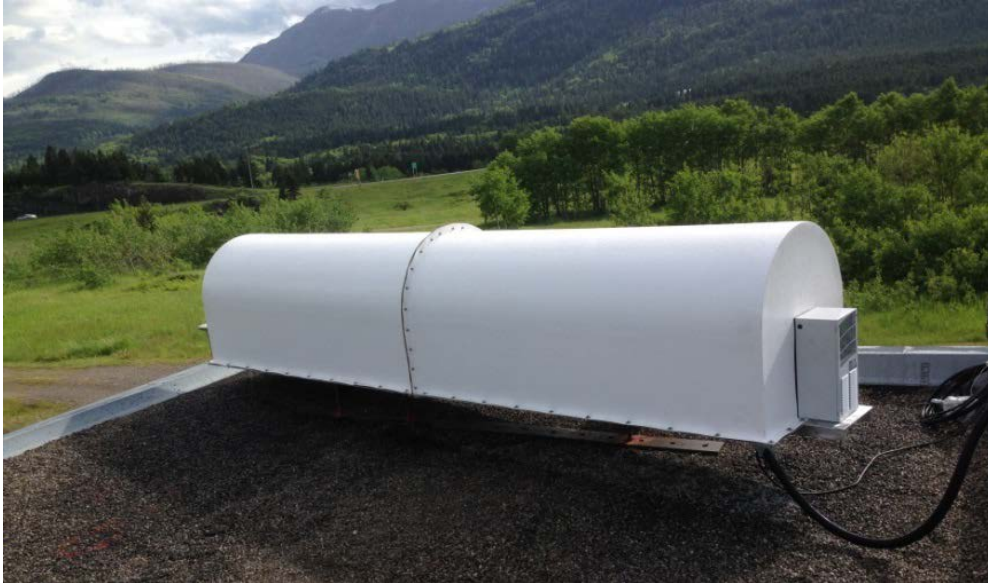
Figure 3. (a) LiSAMobile system without radome and temperature regulation unit; (b) LiSAMobile system completely assembled (Photo courtesy of Ellegi).
