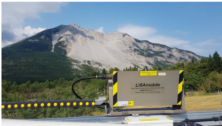
Figure 6. LiSAmobile system without radome (housing structure), Turtle Mountain, Alberta.
