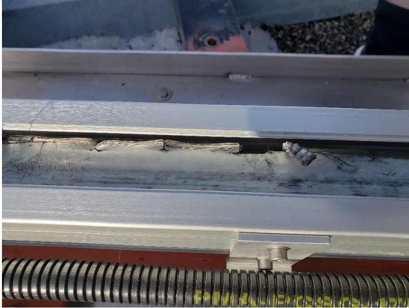
Figure 3. Linear positioner (drive belt) connected to the radar unit was misaligned and damaged, preventing the radar unit from moving along the track of the LiSAmobile unit at Turtle Mountain, Alberta.
