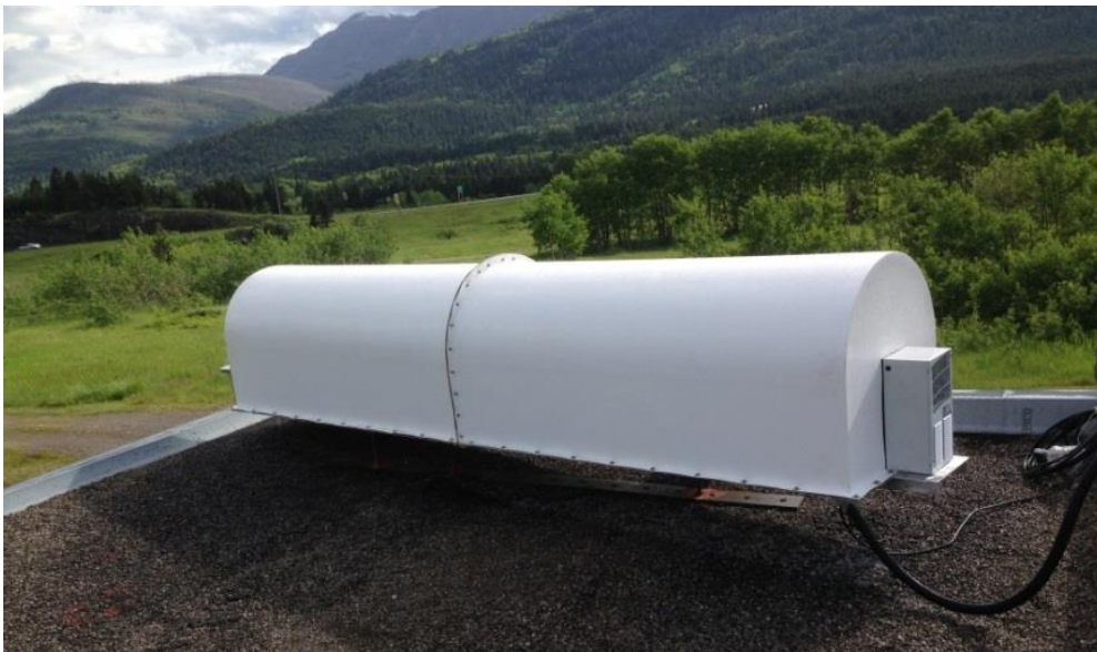
Figure 3. a) LiSAmobile system without radome and temperature regulation unit; b) LiSAmobile system assembled with the radome.
