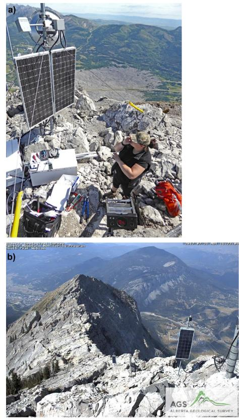
Figure 2. a) Replacement of the South Peak web camera. b) Image from the new South Peak web camera.
