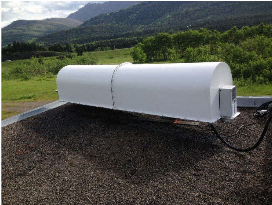
Figure 4. (a) LiSAmobile system without radome and temperature regulation unit; (b) LiSAmobile system completely assembled (Photos courtesy of Ellegi).
