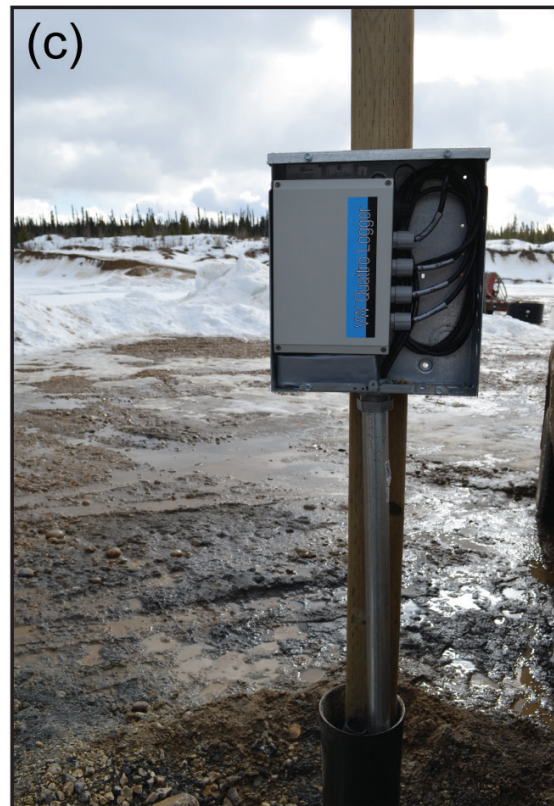
Figure 2. (a) Drill rig and AGS field trailer at site AGS-WCAB15-03; (b) Vibrating wire piezometer attached to tremie pipe; (c) Data logger installation at site AGS-WCAB15-02.
