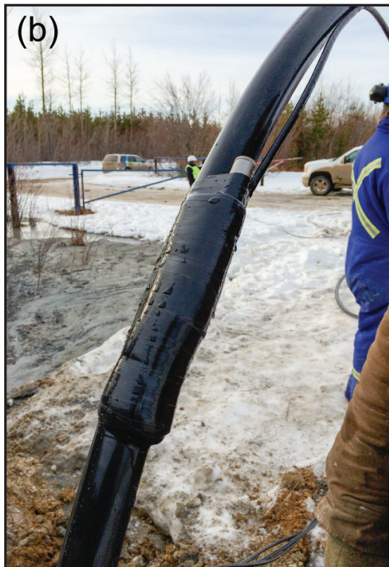
Figure 2. (a) Drill rig and AGS field trailer at site AGS-WCAB15-03; (b) Vibrating wire piezometer attached to tremie pipe; (c) Data logger installation at site AGS-WCAB15-02.
