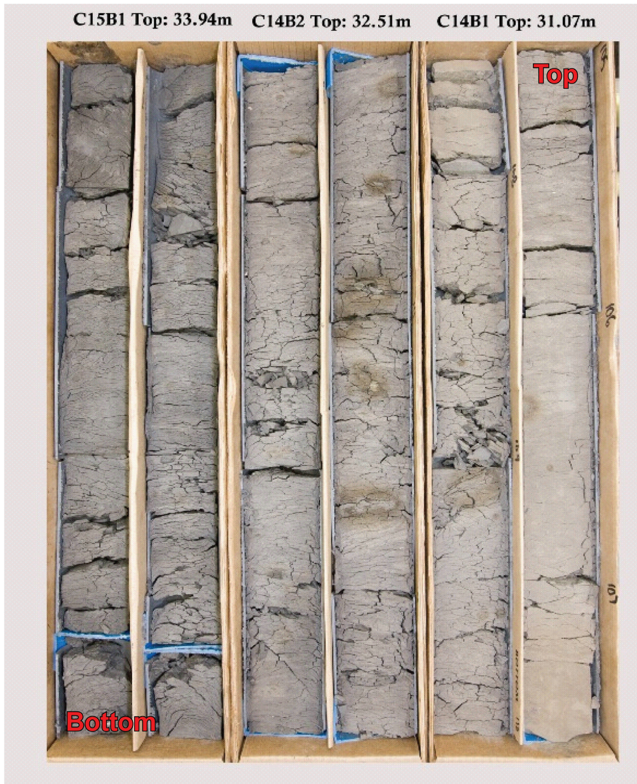
Figure 19. Core photo of lower Clearwater shale from well AA/14-29-095-12W4/0; depth 31.07 m to 33.94 m. (Photo by M. Shepley.)
