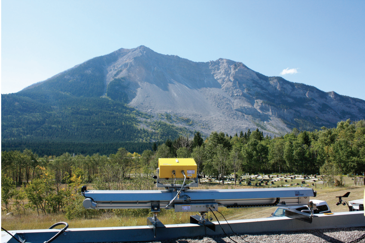
Figure 15. The IBIS system installed in front of Turtle Mountain. The maximum distance from the radar head to the furthest point on the mountain face is about 2.9 km.
