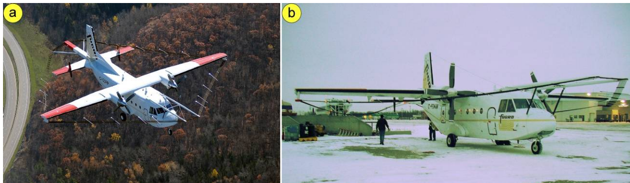
Figure 4. a) The GEOTEM ® survey technique in flight. Note the transmitting loop fixed to the aircraft's nose, tail and wing tips. Primary electromagnetic pulses are created by a series of discontinuous sinusoidal current pulses and transmitted into the transmitting loop. b) Modified Casa 212 aircraft used by Fugro Airborne Surveys in this study.
