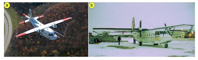
Figure 4. a) The GEOTEM® survey technique in flight. Note the transmitting loop fixed to the aircraft's nose, tail and wing tips. Primary electromagnetic pulses are created by a series of discontinuous sinusoidal current pulses and transmitted into the transmitting loop. b) Modified Casa 212 aircraft used by Fugro Airborne Surveys in this study.
