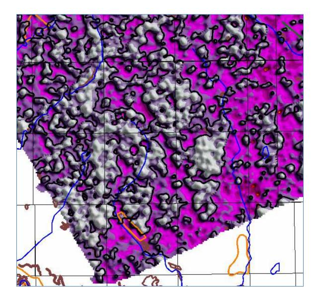
Figure 38: Shaded relief image of the first layer resistivity with the AGS features overlain in the SW corner of the area. The 100 ohm-m resistivity contours in black line are overlain.
