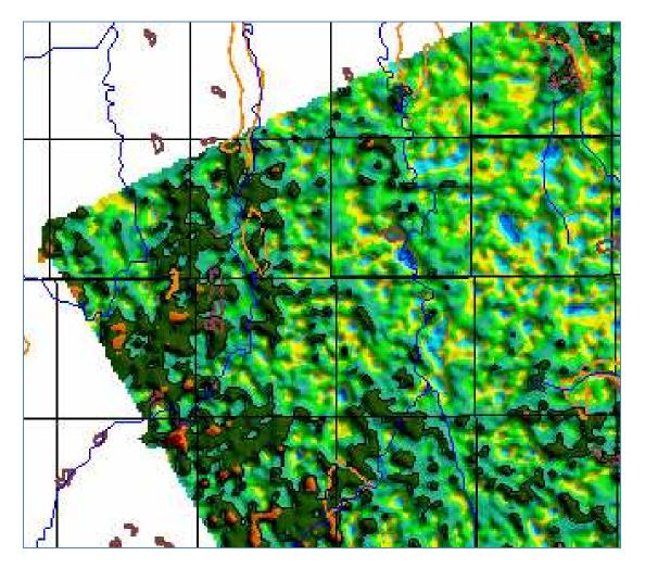
Figure 42a: Shaded relief image of the third layer resistivity with the AGS features overlain in the NW corner of the survey area. Black contours are overlain at a 30 ohm-m level.
