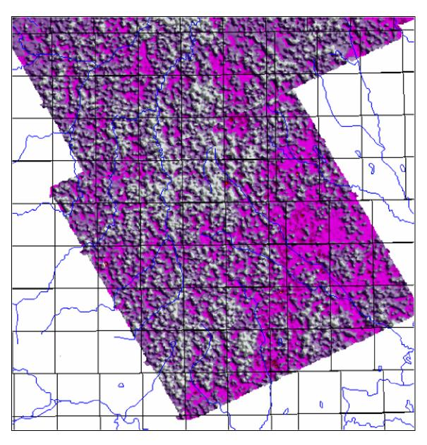
Figure 34a: Shaded relief image of the first layer resistivity across the boundary with the survey to the north.
