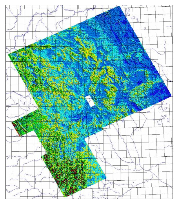
Figure 27: The rnn4, fourth layer resistivity, merged for the current and previous GEOTEM<sup>TM</sup> surveys
