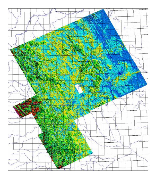
Figure 31: The Thnn3, thickness for third layer, merged for the current and previous GEOTEM<sup>TM</sup> surveys
