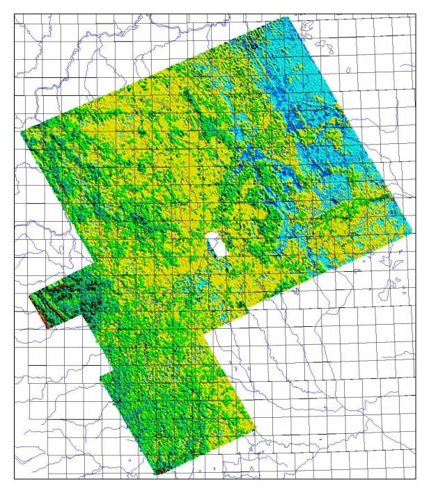
Figure 29: The Thnn1, thickness for the first layer, merged for the current and previous  ${\sf GEOTEM}^{\sf TM}$  surveys
