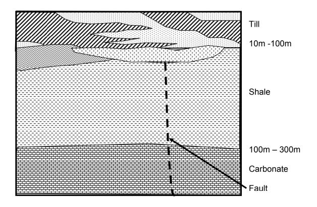
Figure 12b: A cartoon of the possible subsurface geology of the survey area. The model shows till over Cretaceous bedrock shale.
