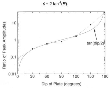
Fig. 6. The ratio of the peak amplitudes of the normalized z-component response (left/right) plotted with solid squares. The ratio plots very close to the tangent of half the dip angle  $\theta$  of the plate.
