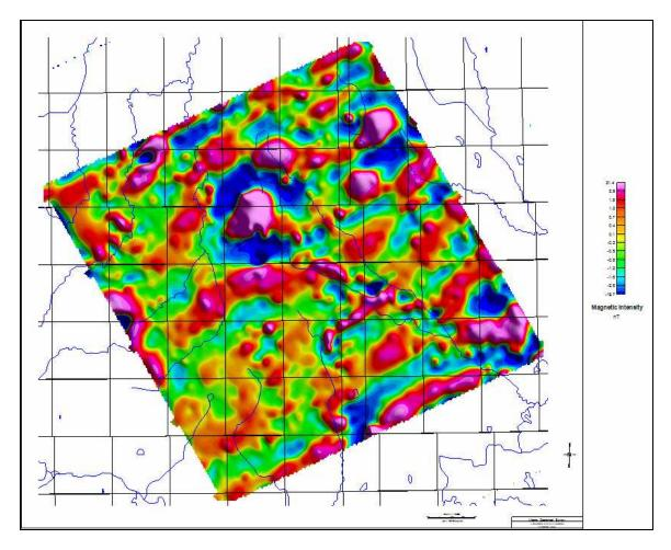
Figure 45b: Band pass filer of the total magnetic field reduced to the pole 2 km to 10 km (Bp 1: 2-10 k).
