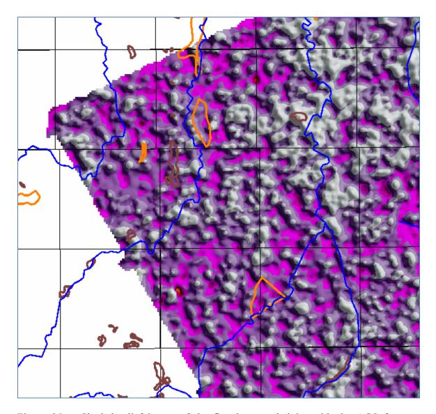
Figure 35: Shaded relief image of the first layer resistivity with the AGS features overlain in the NW corner of the survey area. Black contours are overlain at a 100 ohm-m level.
