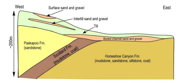
Figure 3. Simplified, regional-scale cross-section, oriented west to east, of sediments and bedrock surveyed using the low-frequency, GEOTEM® time-domain survey, central Alberta.
