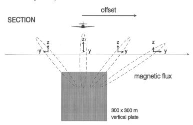
Fig. 12. A sc hematic diagram of the pl ate and the magnetic flux of the secondary field (section view). For increasing offset of the aircraft and receiver from the center of the pl ate, the magnetic field at the receiver rotates from the z to the y component.
