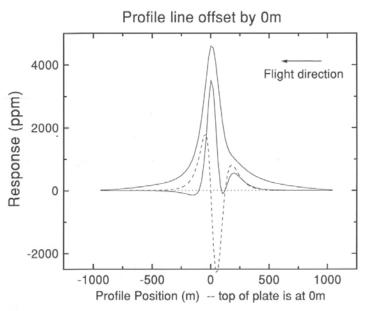
Fig. 9 The response of a 300 by 300 m plate traversed by a profile line crossing the center of the plate in a direction perpendicular to the strike of the plate (the strike angle  $\zeta$  of the plate with respect to the profile line is 90°).
