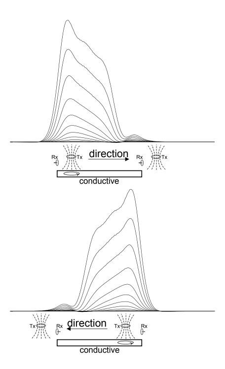
Figure 1. Illustration of how the x-component response varies depen ding on the flight direction. When the receiver flies onto the conductor, the transmitter is over the conductor and current is induced in the conductive material, resulting in a large response. When the receiver flies off the conductor, the transmitter is not over conductive material, so the response is small.
