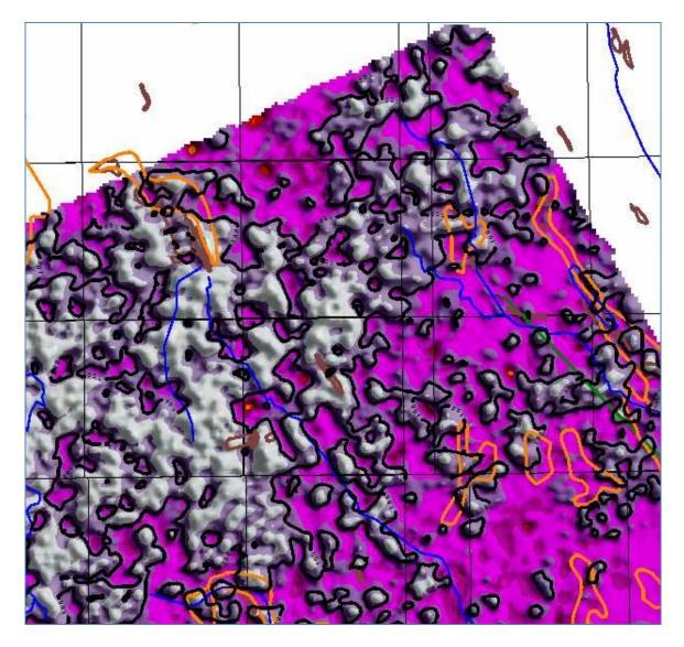
Figure 36: Shaded relief image of the first layer resistivity with the AGS features overlain in the NE part of the survey area. The 100 ohm-m resistivity contours are overlain, black lines.
