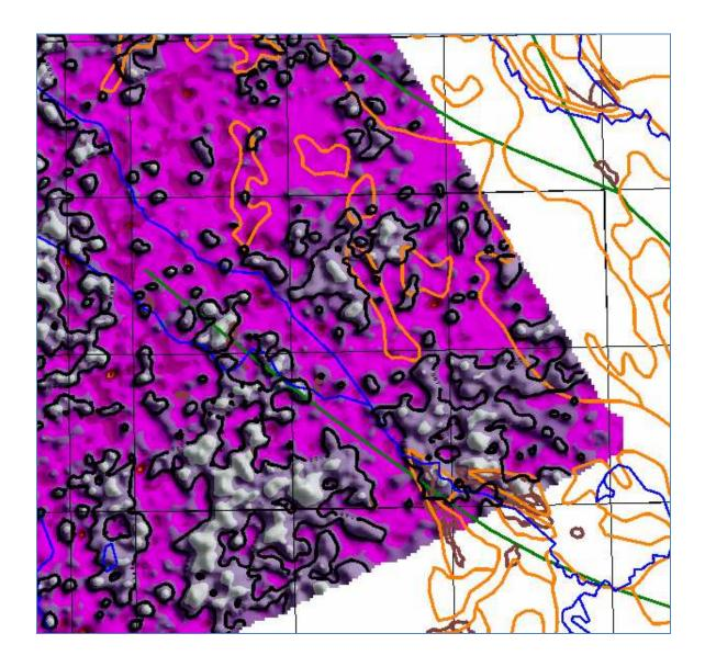
Figure 37: Shaded relief image of the first layer resistivity, rnn1, with the AGS features overlain in the SE corner of the survey area. The 100 ohm-m resistivity contours in black lines overlain.
