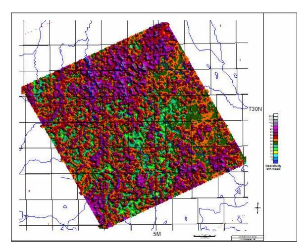
Figure 14a: Shaded relief image of the second layer resistivity, Rnn2.
