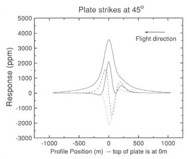
Fig. 11 Same as Figure 9, except the profile line traverses the plate such that the strike angle  $\zeta$  of the plate with respect to the profile line is 45°.
