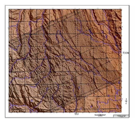
Figure 2: An image of the flight line pattern for the survey. The township and range grid and major drainage is overlain. The image co-ordinates are in the Alberta TM10 projection. The underlying image is the SRTM 90 topographic data.
