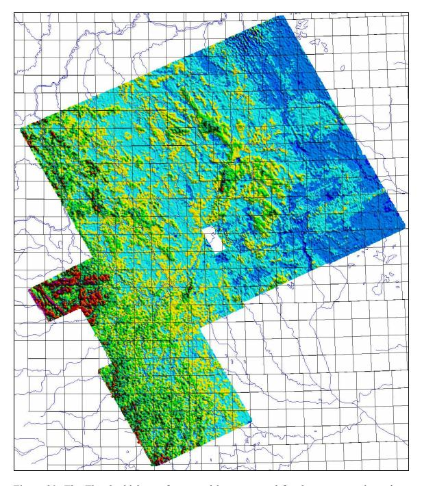
Figure 30: The Thnn2, thickness for second layer, merged for the current and previous GEOTEM<sup>TM</sup> surveys
