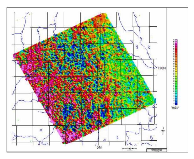
Figure 15b: Shaded relief image of the third layer resistivity, Rnn3, rainbow palette
