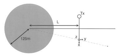
Fig. 16. Plan view of a flat-lying conductor (a circular loop with a radius of 125 m). The AEM system is offset a distance *L* from the center of the conductor in a direction perpendicular to the traverse direction. The traverse direction of the system is from the bottom to the top of the figure.
