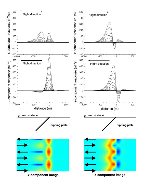
Figure 3. The response over a 45 degree dipping plate. The left panels show the x-component, the right panels the z component. The top is flying left to right, the middle is right to left, the bottom is a plan image with the alternating flight directions shown with arrows.
