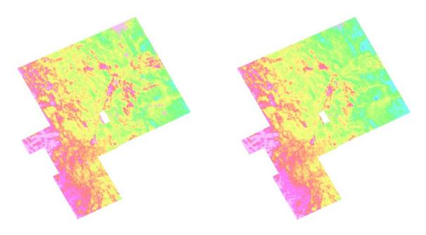
Figure 2. Resistivity Depth Slices at 10 metres (left) and 30 metres (right)
