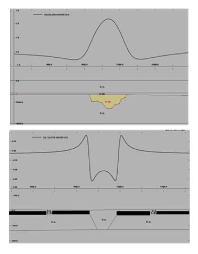
Figure 10: Bottom diagram illustrates the magnetic anomaly characteristics over an outcropping or buried channel cutting a magnetic horizon. The upper diagram is a model result showing the magnetic response of a channel that is magnetic. Note the very different anomaly shape for the two types of magnetic sources.
