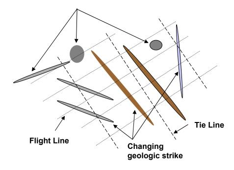
Figure 11: Illustration of aliasing due to flight line spacing
