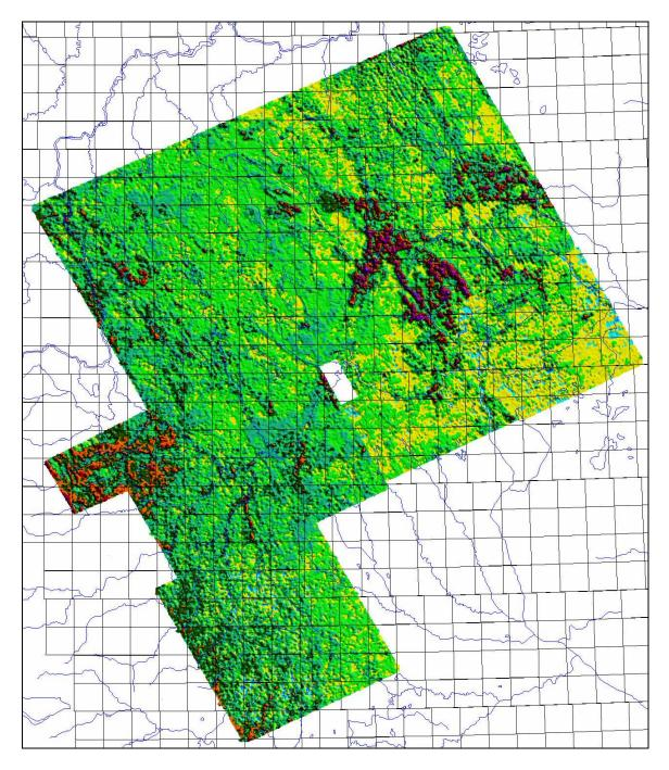
Figure 26: The rnn3, third layer resistivity, merged for the current and previous GEOTEM<sup>TM</sup> surveys
