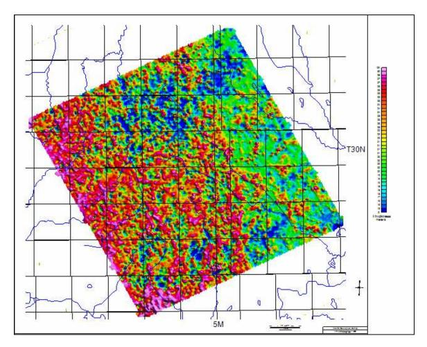
Figure 21b: Shaded relief image of the fourth layer thickness, Thnn4, with a rainbow palette
