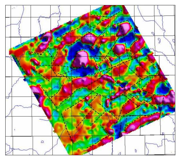
Figure 45c: Band pass filer of the total magnetic field reduced to the pole 2 km to 10km (Bp 1: 2-10k).
