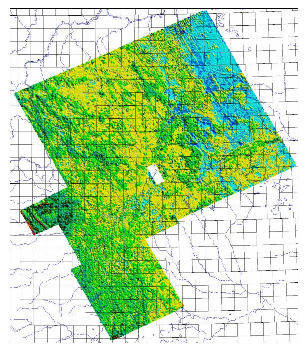
Figure 32: The Thnn4, thickness for fourth layer, merged for the current and previous GEOTEM<sup>TM</sup> surveys
