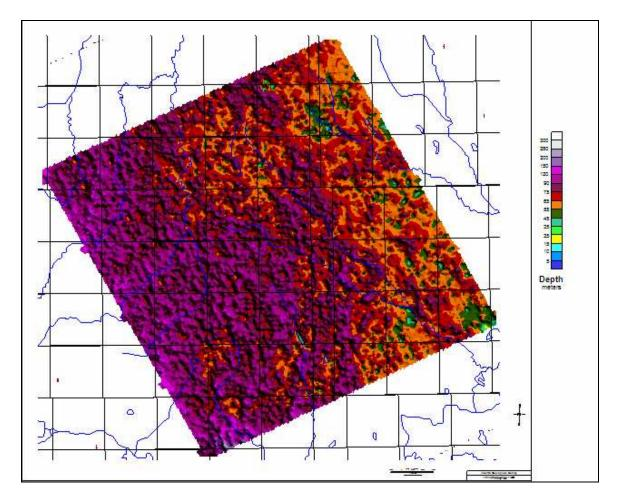
Figure 22 shows the shaded relief image of the total thickness of the four layers, or the depth to the fifth layer, the deepest layer or half space resolved in the inversion process, Figure 4.
