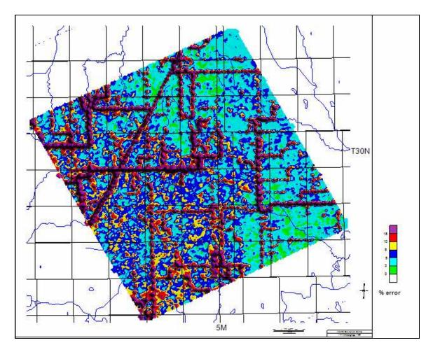
Figure 23 shows the shaded relief image of the least square error of fit for the nn model.
