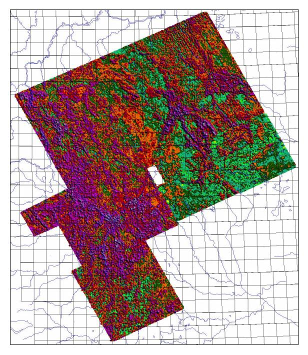
Figure 25: The rnn2, second layer resistivity, merged for the current and previous GEOTEM<sup>TM</sup> surveys.
