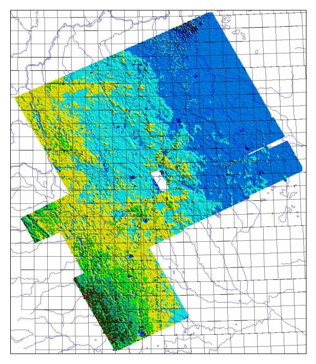
Figure 28: The rnn5, resistivity for fifth layer, merged for the current and previous GEOTEM<sup>TM</sup> surveys
