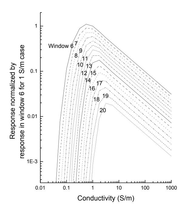
Figure 16. Nomogram for windows 6-20 normalized to a response from a 1 Siemen conductor in window 6.
