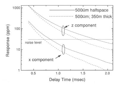
Fig. 2. The response for a 500  $\Omega$ ·m half-space (solid line) and a 500  $\Omega$ ·m layer of thickness 350 m overlying a resistive half-space (dashed line). The z-component responses are the two curves with the larger amplitudes and the two x-component response curves are 6 to 10 times smaller than the corresponding z component. A noise level of 30 ppm is considered to be typical of both components in the absence of strong sferics.
