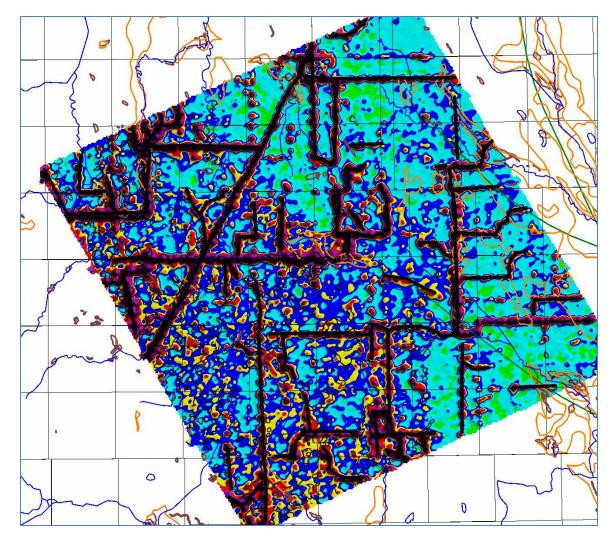
Figure 34b: The per cent error image with the high resistivity features highlighted by black lines. Features are likely cultural affects such as pipelines.
