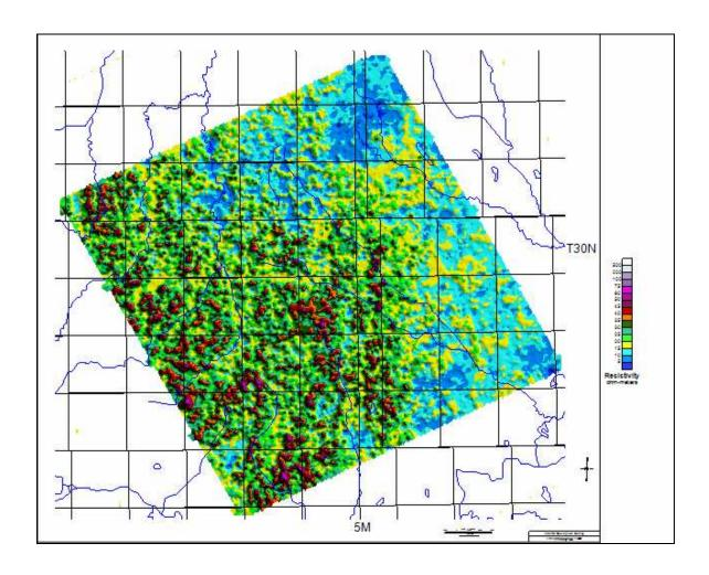
Figure 16a: Shaded relief image of the fourth layer resistivity, Rnn4
