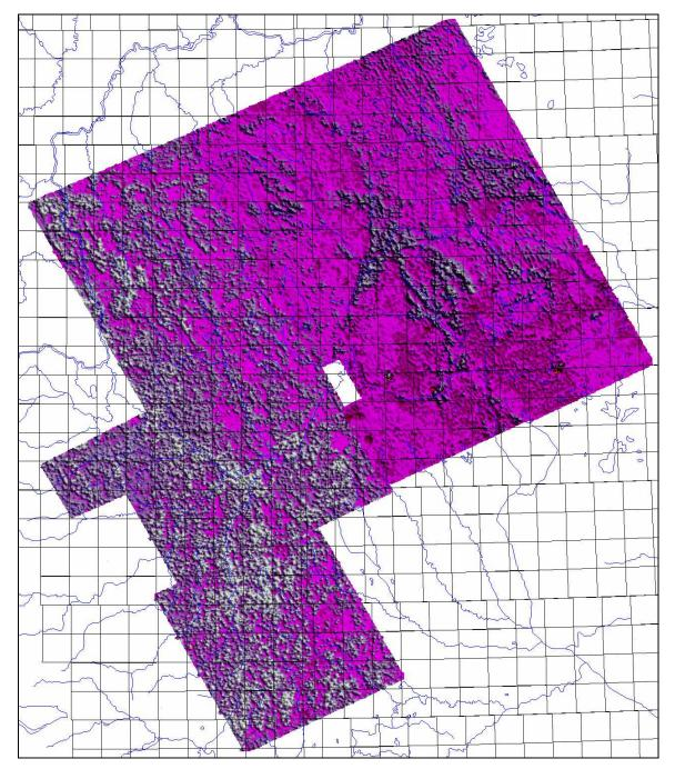
Figure 24: The rnn1, first layer resistivity, merged for the current and previous GEOTEM<sup>TM</sup> surveys.
