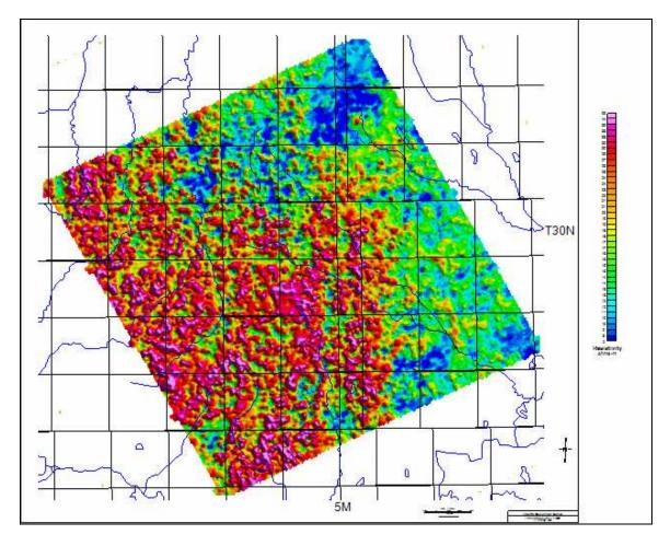
Figure 16b: Shaded relief image of the fourth layer resistivity, Rnn4, with a rainbow palette
