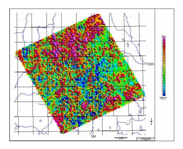
Figure 14b: Shaded relief image of the second layer resistivity, Rnn2, with a rainbow palette.
