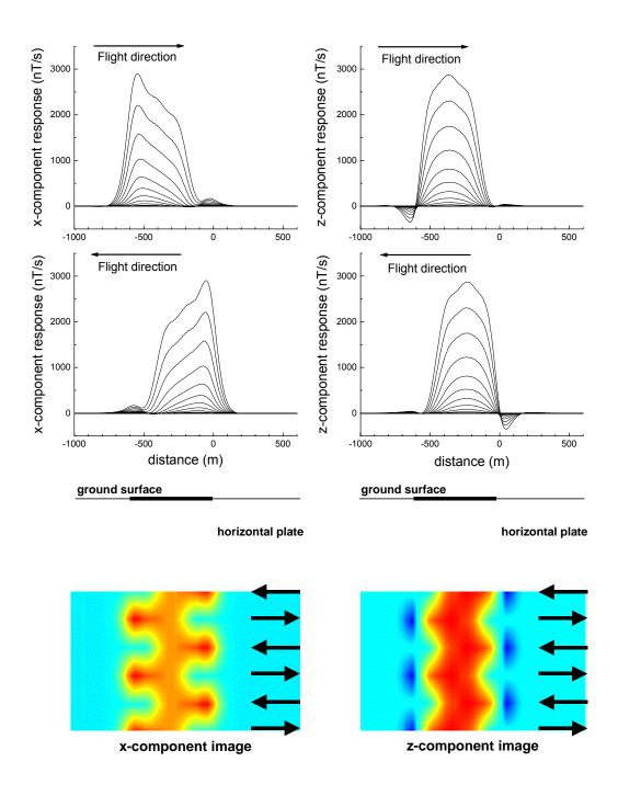
Figure 4. The response over a ho rizontal plate. The left panels sho w the x-component, the right panels the z component. The top is flying left to right, the middle is right to left, the bottom is a plan image with the alternating flight directions shown with arrows.
