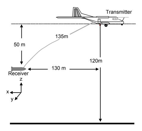
Figure 3. Nominal geometry of the fixed-wing electromagnetic system.
