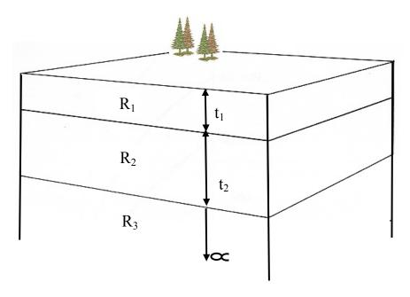
Figure 3: Layered earth model used in the inversion process. The earth may be any number of layers, but typically is six or less. The layer parameters found by inversion are each of the layer resistivities, R, and thicknesses, t. The lowermost layer is "infinite".
