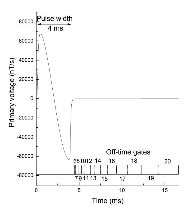
Figure 2. Theoretical transmitter waveform response in the receiver.
