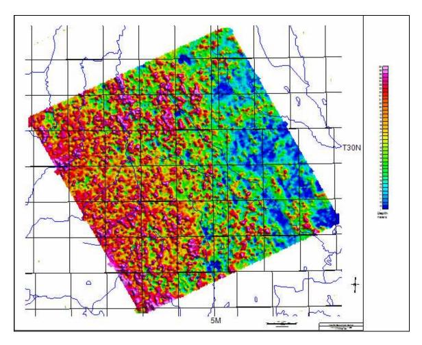
Figure 18b: Shaded relief image of the first layer thickness, Thnn1, with a rainbow palette.
