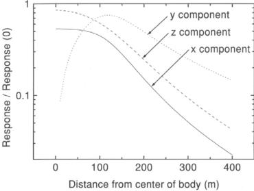
Fig. 17. The normalized response of the EM system plotted as a function of increasing offset distance L. The x component falls off most rapidly and the y component most slowly with increasing offset distance.
