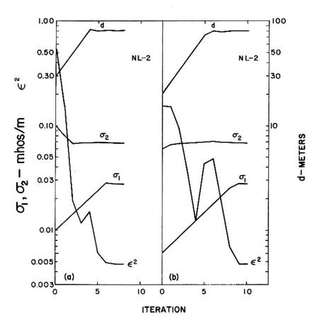
Figure 6: Figure shows the changing conductivity, σ, (inverse of resistivity) and first layer thickness, d, with iteration for a two layer model. The least square error, ε, is also shown. The left and right views show the iterative process converge to nearly identical models starting with different starting values for the two layer conductivities and the first layer thickness (After Glenn et al., 1973).
