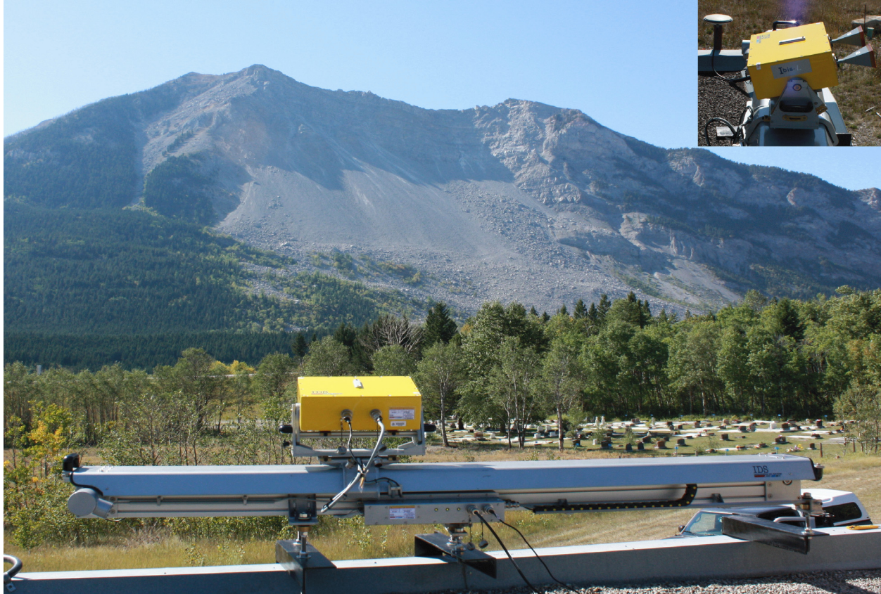
Figure 14. The IBIS-L GB-InSAR system is installed on a rooftop, facing unstable slopes on Turtle Mountain. The farthest point on the mountain crest is approximately 3200 m away.
