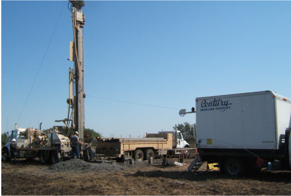
Figure 4. Century Wireline Services conducting downhole geophysical logging at one of the ECC boreholes.
