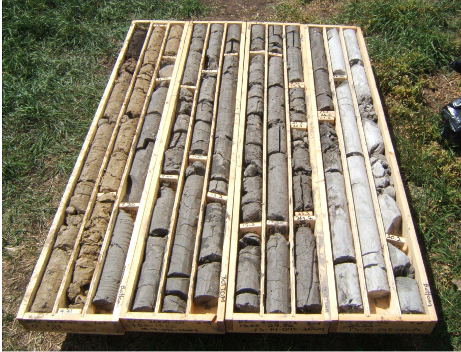
Figure 5. Core boxes used to store and transport recovered core. Top of hole is in the upper left corner.
