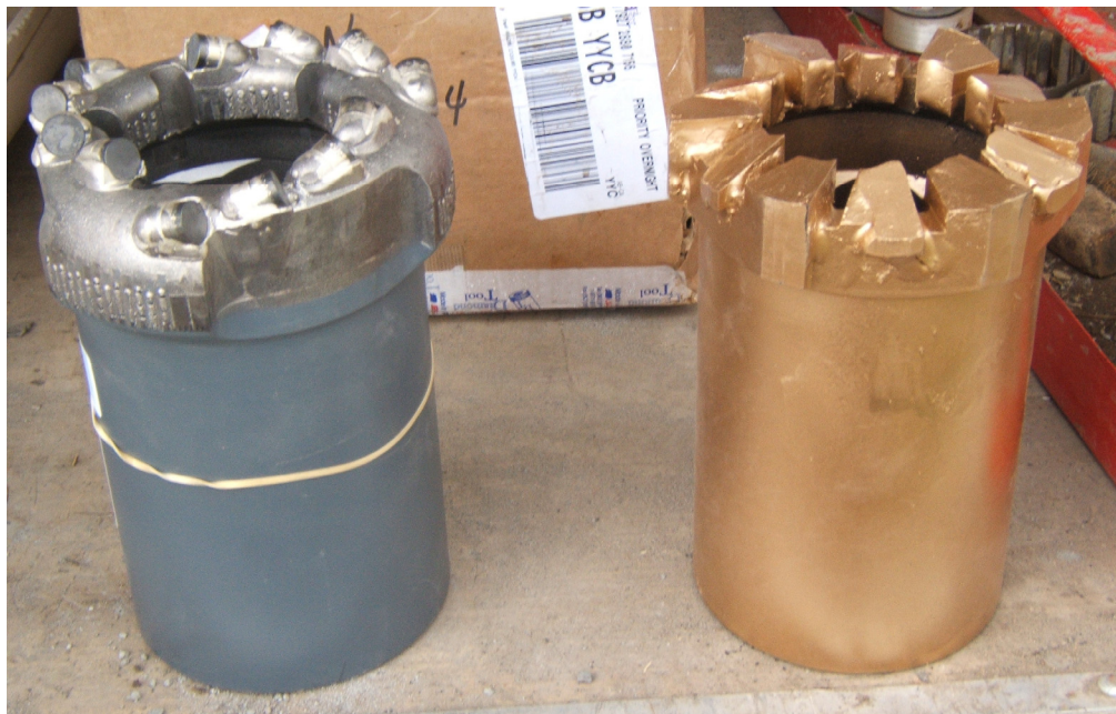
Figure 3. Bit types used for the drilling program: STRATAPAC™ diamond bit (left) and carbide-tipped bit (right).
