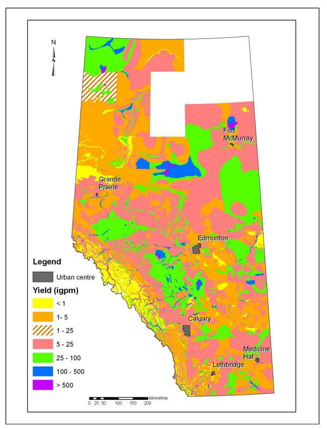
Figure 4. Compilation of water-well yields. Abbreviation: igpm, imperial gallons per minute.
