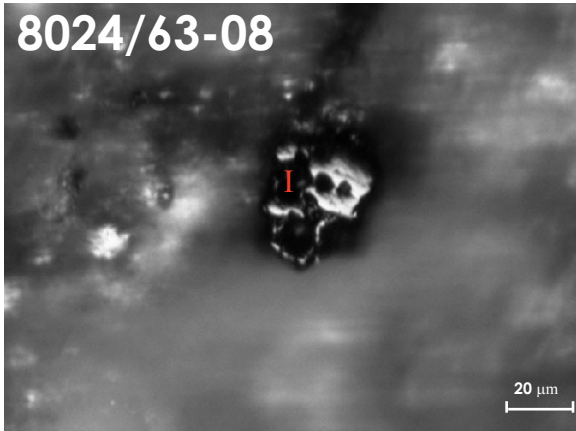
8024/63-08. Pyrite-rich shale with lenses of weak yellow to orange-fluorescing fluoramorphinite (F) with yellow-fluorescing alginite (mostly Prasinophyte (P) and liptodetrinite) inclusion, weak orange-fluorescing bitumen (B) and bright yellow-fluorescing bitumen. Also contains reworked vitrinite and inertinite (I) maceral. Fluorescent and reflected white light.
