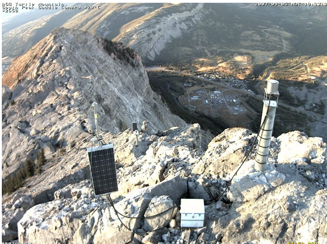
Figure 9. Image from the web camera on the South Peak of Turtle Mountain. Photo: H. Bland, Pinnacle Technologies (Alto Instruments Ltd.).
