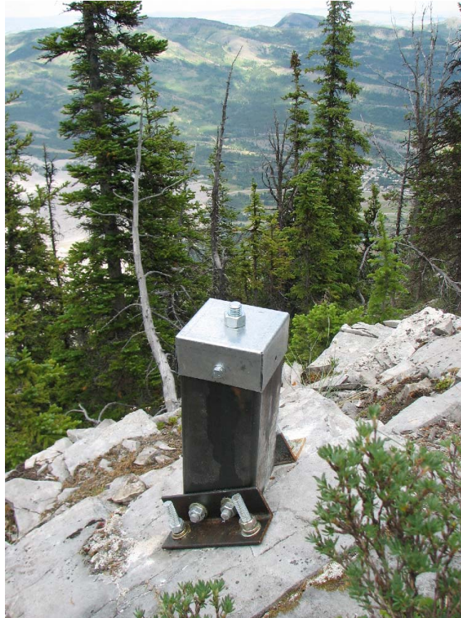
Figure 35. Typical periodic GPS point installation on Turtle Mountain.
