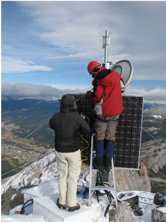
Figure 8. Web camera installation on the South Peak of Turtle Mountain, showing radio antenna, battery boxes and solar panels (left), and close-up of camera, pole mount and mast extension (right). Photo: H. Bland, Pinnacle Technologies (formerly Alto Instruments Ltd.).
