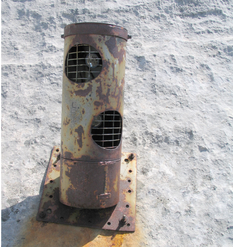
Figure 14. EDM target installed on Turtle Mountain in 1982.
