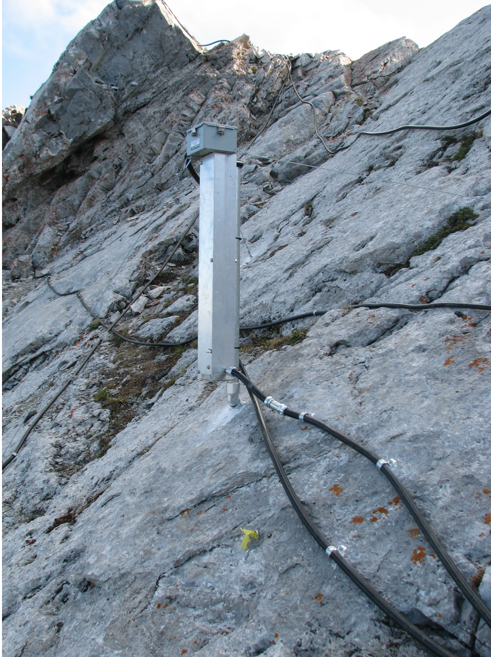
Figure 4. Head assembly for extensometer EX-5.
