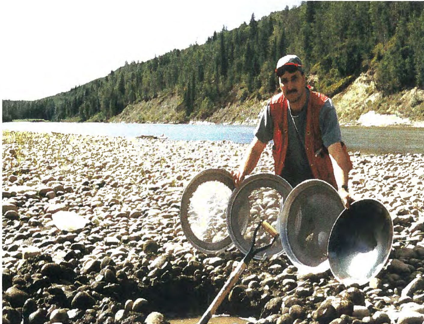
Figure 3. Conical pan and screens used for heavy mineral stream sediment sampling.
