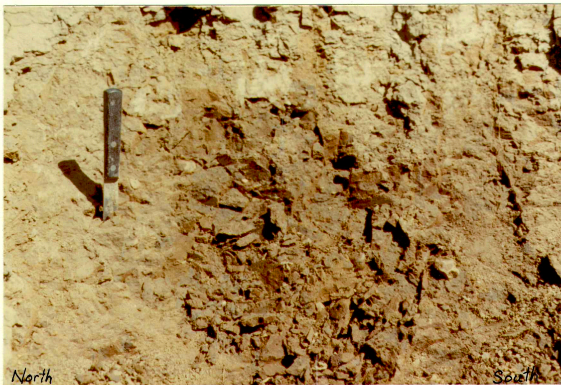
Plate 1d. Fractured, strongly jointed structure of top of Unit 4 till. Note iron and manganese staining along fracture planes.
