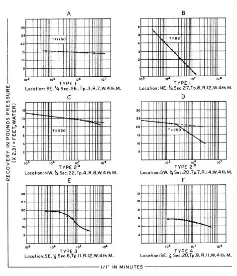
FIGURE 14. Recovery curves of flowing wells
