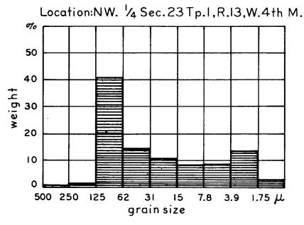
FIGURE 13. Histogram showing grain-size distribution of shale underlying Milk River sandstone
