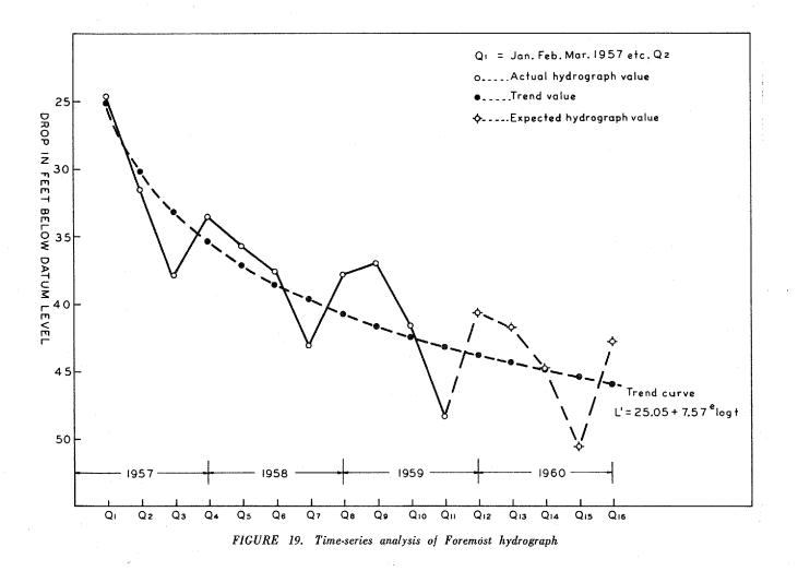
The trend equation was obtained by fitting the curve of equation (7) to the hydrograph data, using the principles of the least squares. The least squares were determined by the normal forms:
