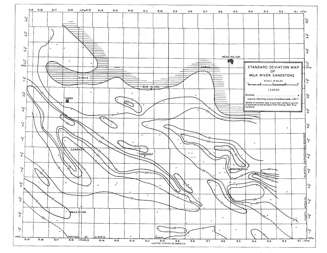
it is necessary to supplement the vertical variability pattern map with sand to shale ratio values, in order to show not only the positions of the sandstone beds, but also the nature of the section at any particular locality. There appears to be good correlation between the nine classes and the sand to shale ratios. The two variables and the sand to shale ratios for the Milk River sandstone were calculated for 160 electrologs and the results are shown in figure 10.
