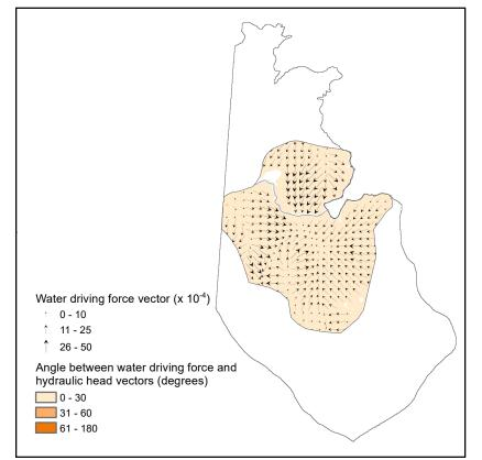
Figure 5. Water driving force vector map of the Dunvegan HSU. The map only covers the area where hydraulic head and TDS gridded surfaces overlap.
