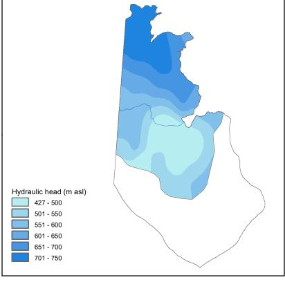
Figure 4. Distribution of hydraulic head in the Dunvegan HSU (Singh and Lemay, 2021). The map extent is based on the spatial distribution of hydraulic head data and differs from the extent of the main map.
