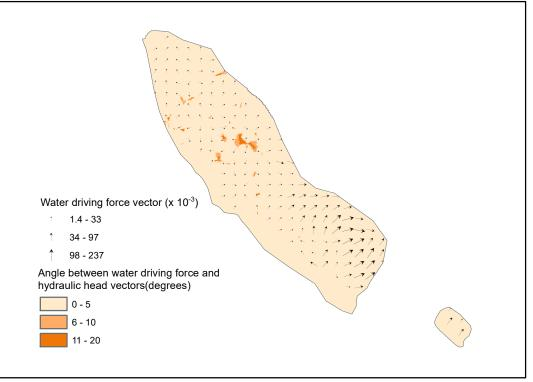
Figure 6. Water driving force vector map of the Cardium HSU. The map covers only the area where hydraulic head and TDS gridded surfaces overlap.
