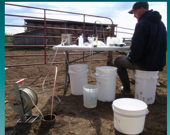
Landon Wood (Alberta Geological Survey summer student) processing water samples collected in the central portion of the ECC. Water samples are collected for different types of analysis. The collection protocols for each sample type are carefully developed to avoid contamination during sampling. Landon is wearing gloves to not contaminate the sample, and the sampling materials are relatively inert to not contaminate the sample during collection.
