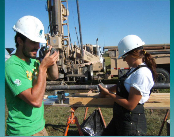
Josh Bishop and Elizabeth Kravontka (Alberta Geological Survey summer students) examining core at a drill site. They are examining the size of the grains in the samples. Important aspects to consider when examining core include the type of sediment encountered, its colour and the thickness of the material.
