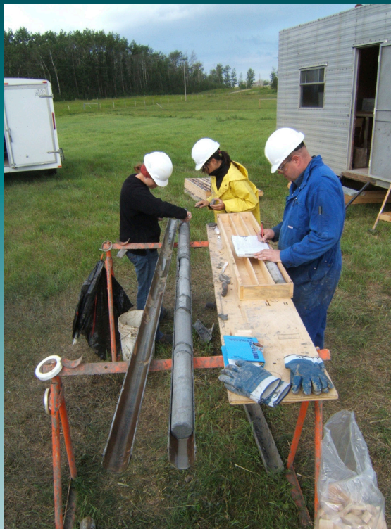
Alyssa Barker, Alberta Environment, Joanna Chan, (Alberta Geological Survey summer student) and Tony Lemay, Alberta Geological Survey, logging core for the ECC borehole-drilling program. Rocks of the Horseshoe Canyon Formation are being described. The Horseshoe Canyon Formation contains many different rock types, including sandstone, siltstone, mudstone and coal. This core in particular contained abundant finer grained sandstone.
