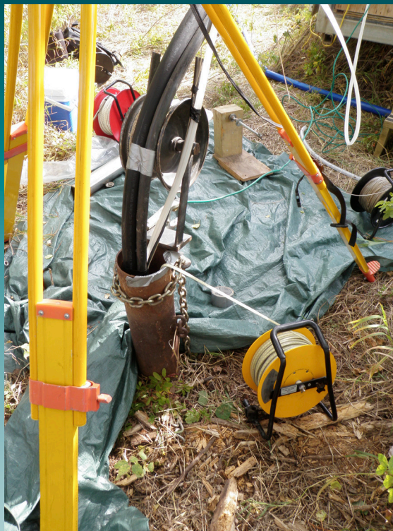
The Alberta Geological Survey sampling team visited a site in conjunction with Alberta Environment. The equipment inserted into the well includes a submersible pump to conduct a pump test, a water-level tape to measure the water level and sampling tubing to collect a water sample.
