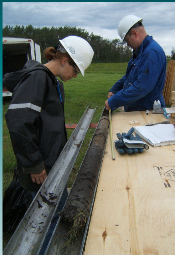
Alyssa Barker, Alberta Environment, and Tony Lemay, Alberta Geological Survey, examine sediments from above bedrock in a core sample. This coring run collected material from the land surface (note the grass) down to approximately 2 m below ground surface. Notice how the colour changes with depth. Information on the colour along with the types of sediment present can tell us about the history of the site.
