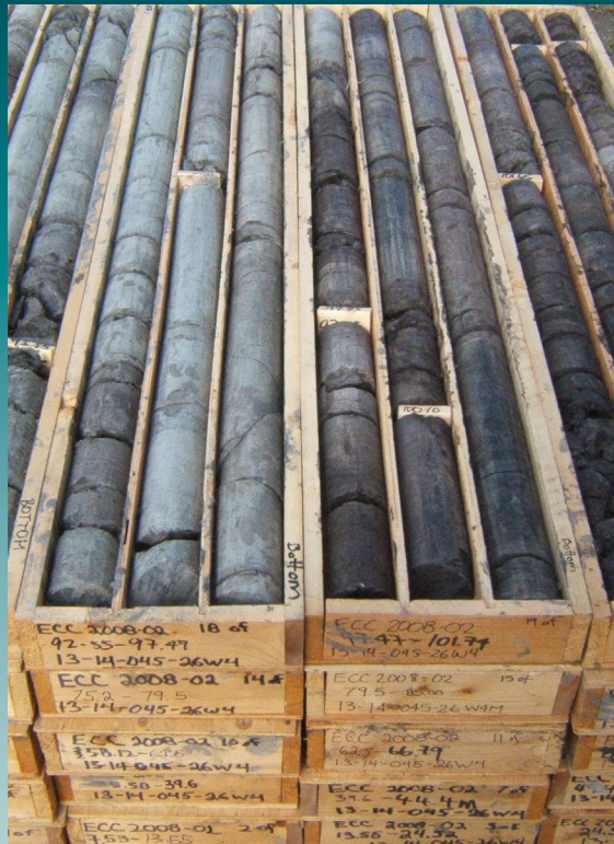
Core samples from the borehole drilling program. The light grey rocks (left) are from the Scollard Formation and consist of mudstone, siltstone and fine-grained sandstone. The dark grey rocks (right) are from the Battle Formation and consist of mudstone. The dark colour and rock type are typical of the Battle Formation.
