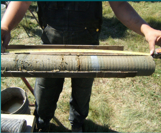
Measuring the thickness of the types of rock material in a core sample. Once a core sample is brought to the surface, the types of sediment or rock material are described, including the thicknesses, their colour and any other important observations that may identify the formation, and the environment in which the materials were deposited.
