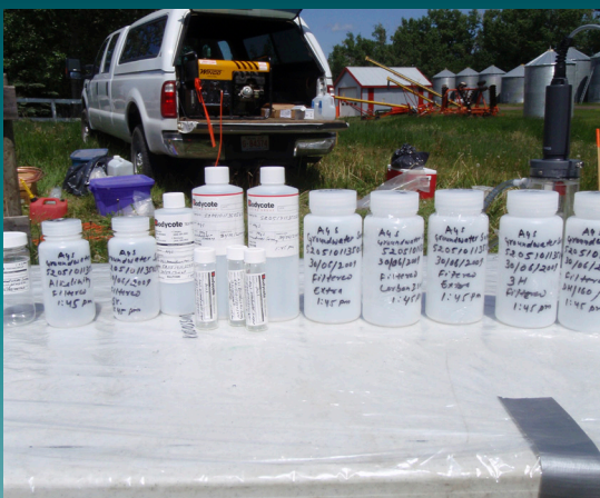
Different samples are collected at each site for different types of analyses. Each analysis has different requirements, including the type of bottle used to hold the sample. This photo shows the various types of bottles used in sampling work.
