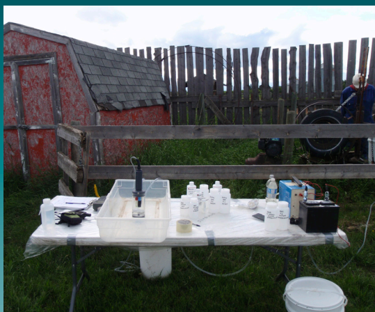
Typical groundwater sampling set up. Prior to sampling, all bottles are labelled, the equipment is connected to a sampling point, or lowered down the well, and any equipment that measures the physical or chemical properties of the water are calibrated.
