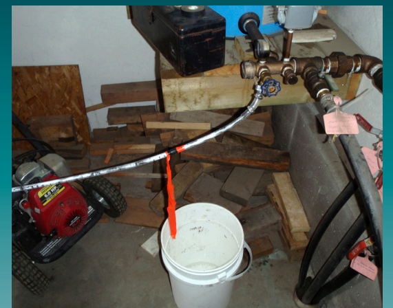
Collecting a water sample from a well with a manifold (upper right). Because of the types of analyses performed on the groundwater samples we collect, it is important for the sample to be collected prior to it entering any pressure tank or treatment system. In this case, the manifold has a connection point prior to the groundwater from the well entering a pressure tank.
