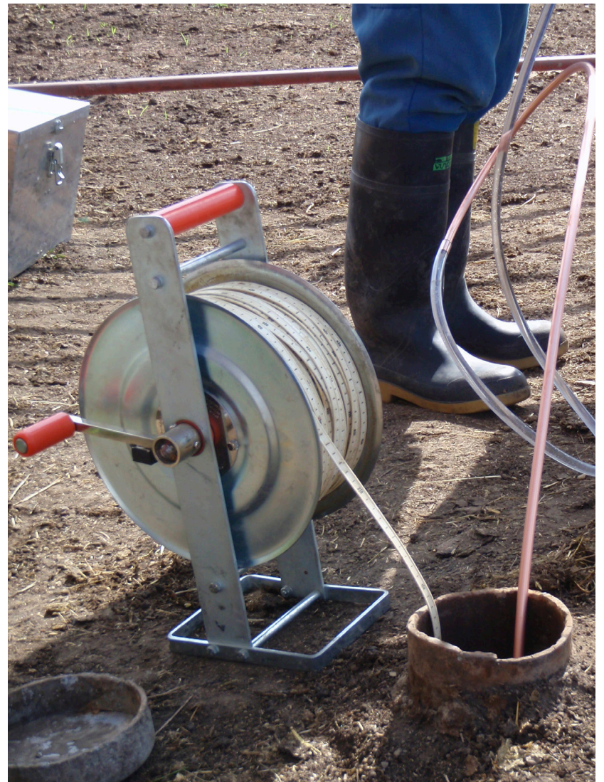
Measuring the water level using a water-level tape and collecting groundwater samples from a well in the central portion of the ECC.
