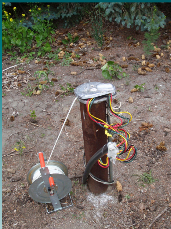
Measuring the water level in a well prior to collecting groundwater samples. The water-level tape is lowered into the well until it touches the water. The depth is determined using the measurement scale on the tape.
