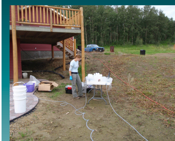
Alyssa Barker, Alberta Environment, collecting groundwater samples from a well in the central part of the ECC. Whereas the sampling protocols remained the same for each site, the geology of potential aquifers would change. The effects of the geological and hydrogeological settings on the hydrochemistry were key questions asked at the outset of the program. Answering these question dictated the details of the sampling program.
