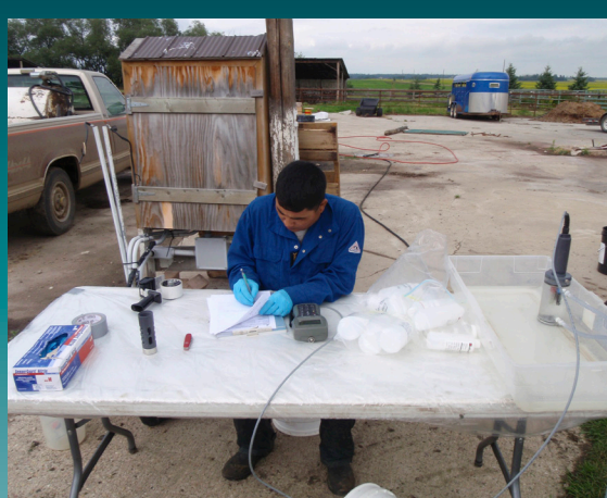
Hira Moktan, Alberta Environment, taking field notes during sampling. The information collected at each site includes site location, site description, physical and chemical measurements (like groundwater pH), and quality control-quality assurance details.
