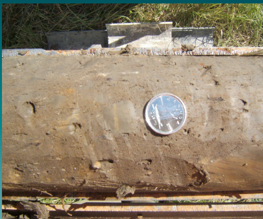
Till sample recovered during the drilling program in the ECC. The coin is included for scale. The till in this instance is light grey-brown with some rusty colouration. The colour is an important tool in mapping the occurrence of till from place to place in the subsurface.
