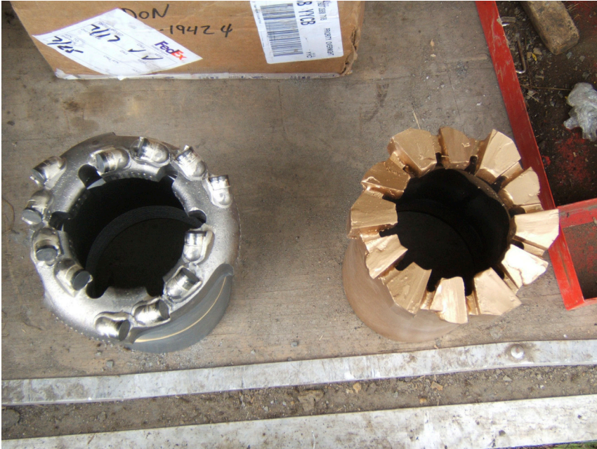
Borehole-drill bits for coring. The silver bit on the left has a diamond-impregnated cutting surface for bedrock coring. The gold bit on the right is for coring unconsolidated sediments above bedrock.
