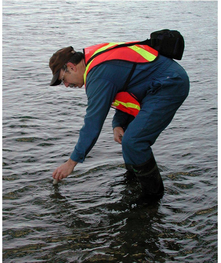
Gordon Jean, Alberta Geological Survey, measuring the physical properties of the water in the North Saskatchewan River near Edmonton, Alberta. Measurements included pH, conductivity, dissolved oxygen and temperature. These water properties are used to report on the water quality in the study area.
