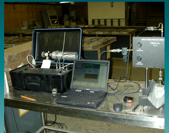
Measuring the permeability of a rock sample collected during the ECC drilling program. A tool called a mini-permeameter determines the permeability of a rock sample by measuring how much nitrogen gas can be injected into the rock over time.
