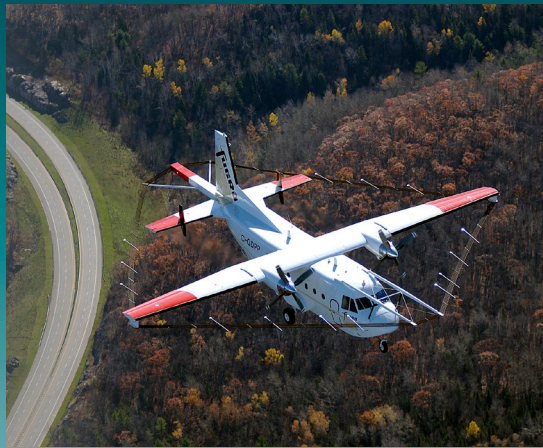
An airplane outfitted with the GEOTEM system to perform airborne geophysical surveys for a portion of central Alberta. Photo courtesy Fugro Data Solutions (Canada) Inc.
