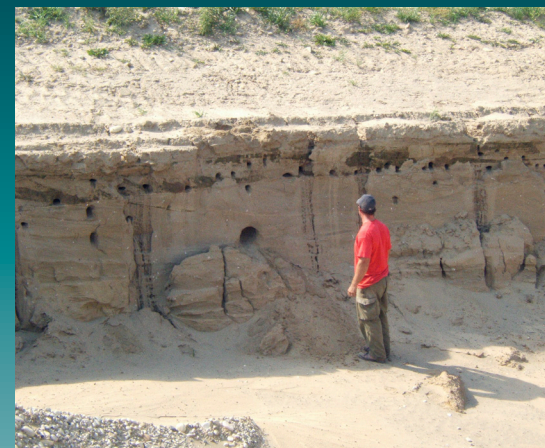
Shawn Slattery, Alberta Geological Survey, examines a fluvial sand exposure. The grain size of the sand and any layering within it can help reconstruct the depositional history of the area. This exposure has many burrows, indicating it is a relatively soft material. However, it has a cliff-like form; therefore, it has some structural strength.
