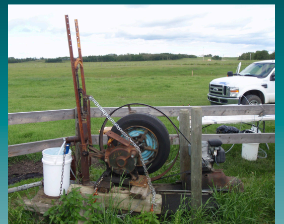
Ingenious design for a well. The pump mechanism uses many different components, including a wheel rim, a tire and a small engine. On the left side, you can see the pump's outflow in the white bucket.
