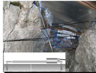
Typical configuration of crackmeters, with aluminum roof mounted to provide protection from snow overburden and falling rocks. Crackmeters were installed in sets of three in order to determine deformation vectors.
