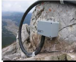
Typical configuration of crackmeters, with aluminum roof mounted to provide protection from snow overburden and falling rocks. Crackmeters were installed in sets of three in order to determine deformation vectors.
