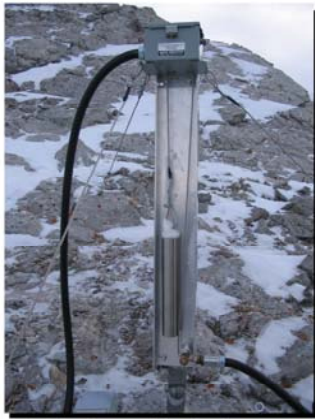
Typical head assembly of a wire extensometer, in which a weighted wire runs over a rotary potentiometer, calibrated to measure millimetres of displacement.
