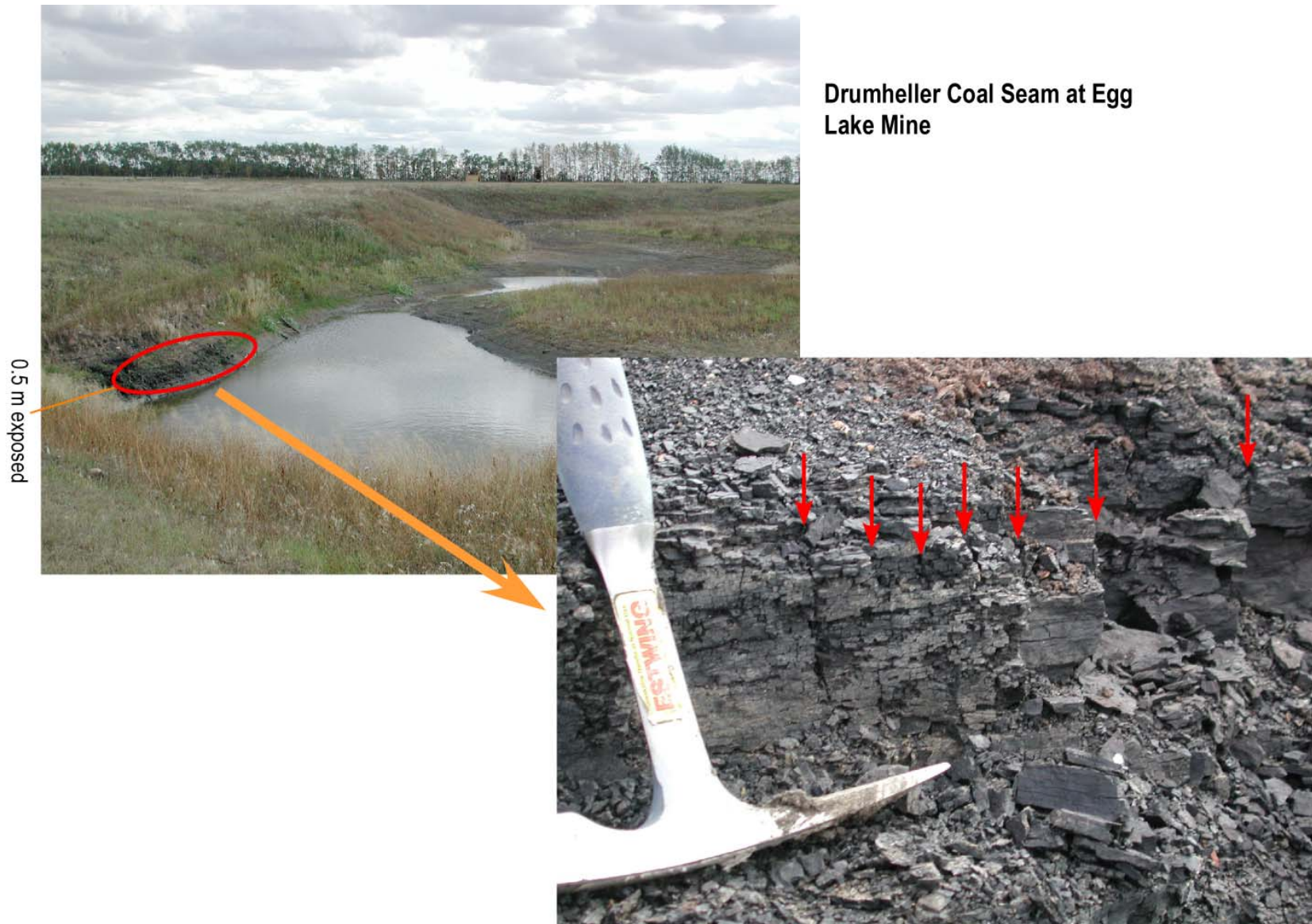
Figure 11. Egg Lake mine site outcrop near Morinville (see Figure 6 for location) showing Drumheller coal seam. Above: Egg Lake mine. Right: Red arrows indicate face cleats, strike N45°E. Butt cleats strike N45°W.
