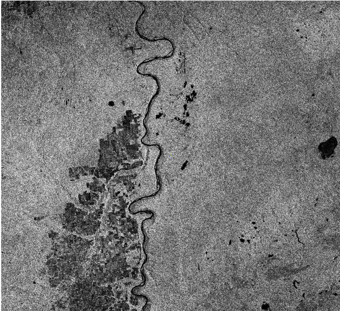
Figure 4. One of the original SGF scene images used for tiling the NTS 84F dataset: scene MO200096 of Standard Beam Mode 7 descending. RADARSAT data © Canadian Space Agency/Agence spatiale canadienne 1999, processed and distributed by RADARSAT International.
