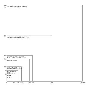
Figure 2. Coverage sizes and resolutions of RADARSAT-1 beam modes (modified after RADARSAT International (RSI), 1999).
