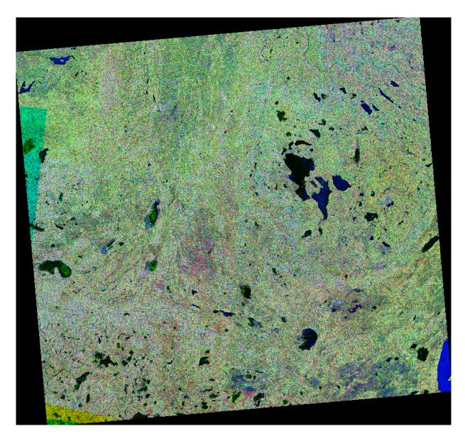
Figure 7. Pseudocolour composite of orthorectified NTS 84B image dataset of Standard Beam Mode S1/S7 ascending/descending beam positions (RGB=S7d, S7a, S1d).
