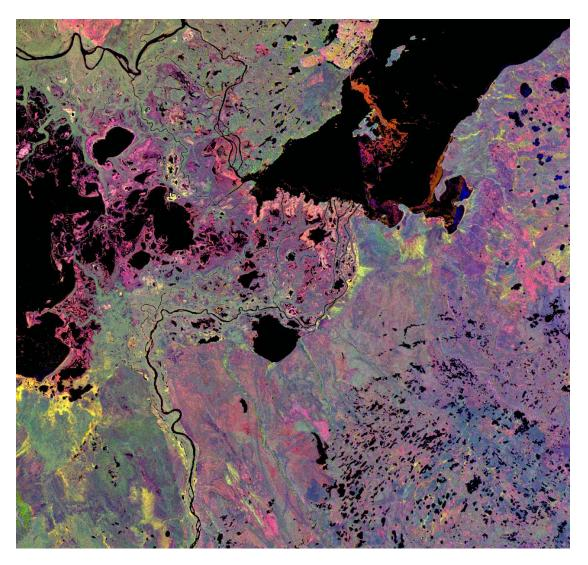
Figure 8. Pseudocolour composite of NTS 74L image dataset of principal component PC1, PC2, PC3 and PC4 (RGB=PC2, PC1, PC3).
