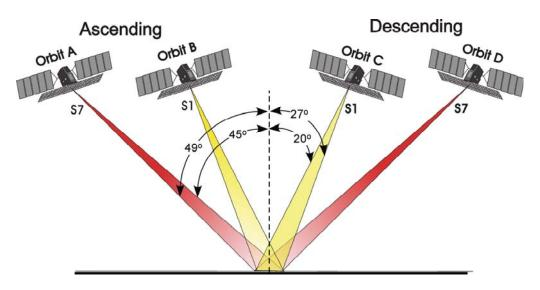
Figure 3. Multi-beam configuration of RADARSAT-1 S1 and S7 ascending/descending imagery (after Grunsky, 2002a).
