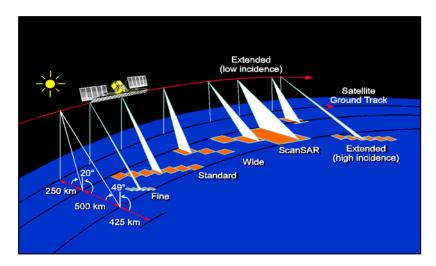
Figure 1. RADARSAT-1 beam modes (used with permision from RADARSAT International (RSI), 1997).
