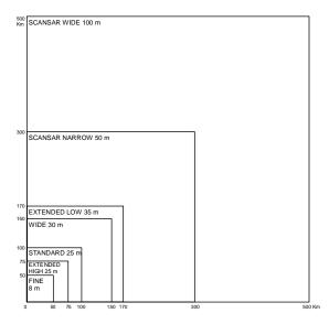
Figure 2. Coverage sizes and resolutions of RADARSAT-1 beam modes (modified after RADARSAT International (RSI), 1999).
