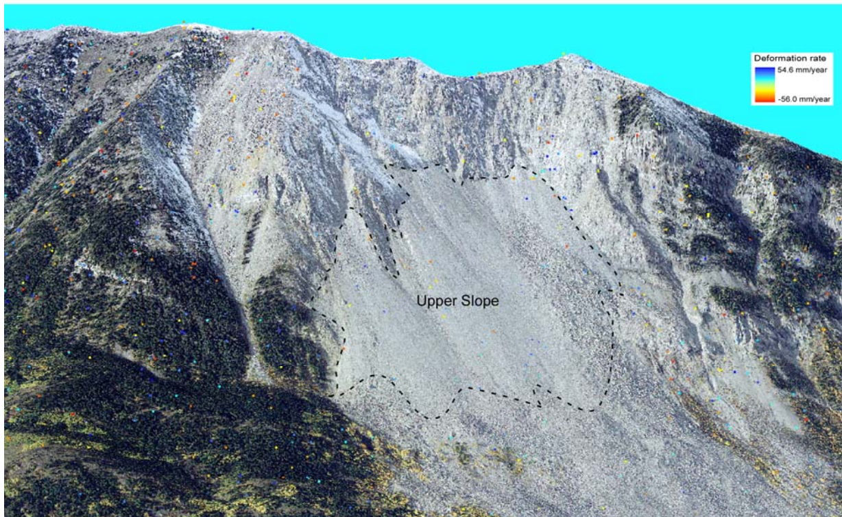
Figure 38. Perspective views to the west of Turtle Mountain–Frank Slide. The upper view simulates the effect of the Fine Beam Mode 4 of the far range. It illustrates that shadow covers much of the upper slope of the Frank Slide.
