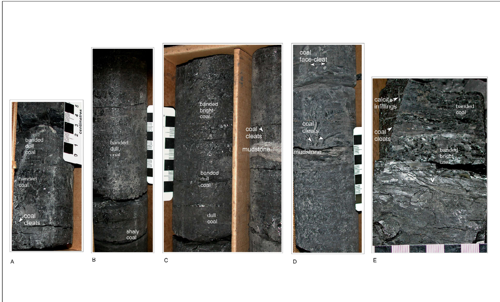
Plate 7. Figure A. Banded coal ((10-27-61-20W5 – 263 m; "M" coal subzone). Figure B. Banded coal ((10-27-61-20W5 – 269 m; "M" coal subzone). Figure C. Banded coal ((10-27-61-20W5 – 295 m; "M" coal subzone).
