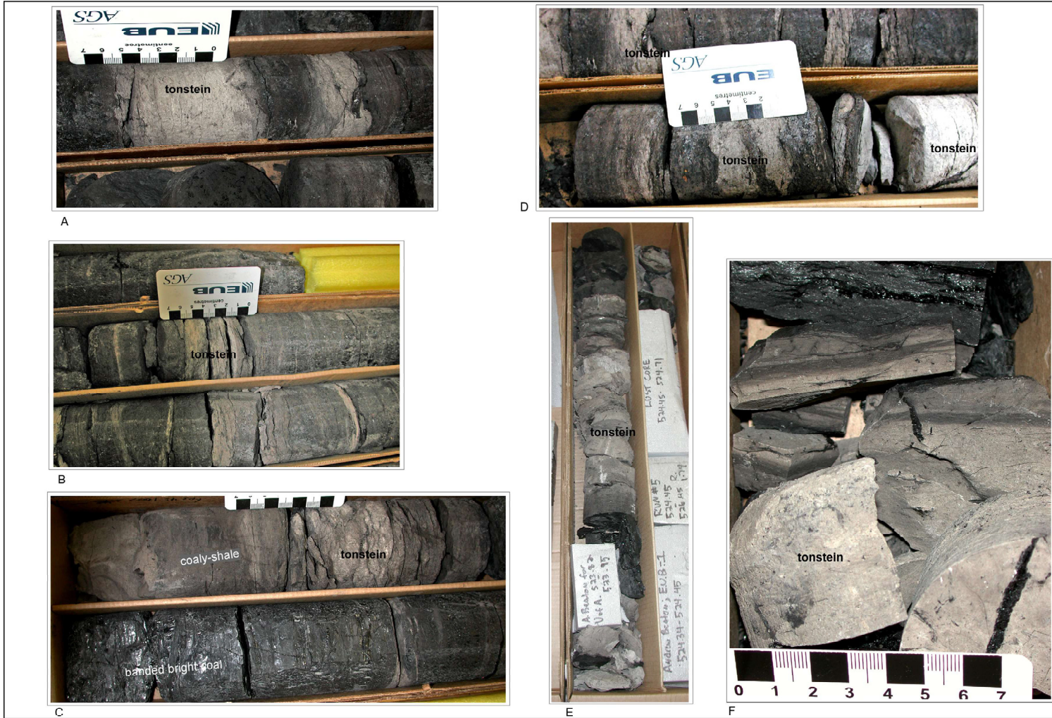
Plate 12. Figure A. Coaly-shale interbedded with tonstein (T) (10-27-61-20W5—260 m). Figure B. Coaly-shale interbedded with tonstein (T) (10-27-61-20W5—263 m). Figure C. Thin bed of tonstein within coal zone (11-06-56-19W5). Figure D. Coaly-shale interbedded with tonstein (T) (10-27-61-20W5—263 m). Figure E. Thin bed of tonstein within coal (11-01-56-19W5—573 m). Figure F. Tonstein: detail (11-01-56-19W5—590 m).
