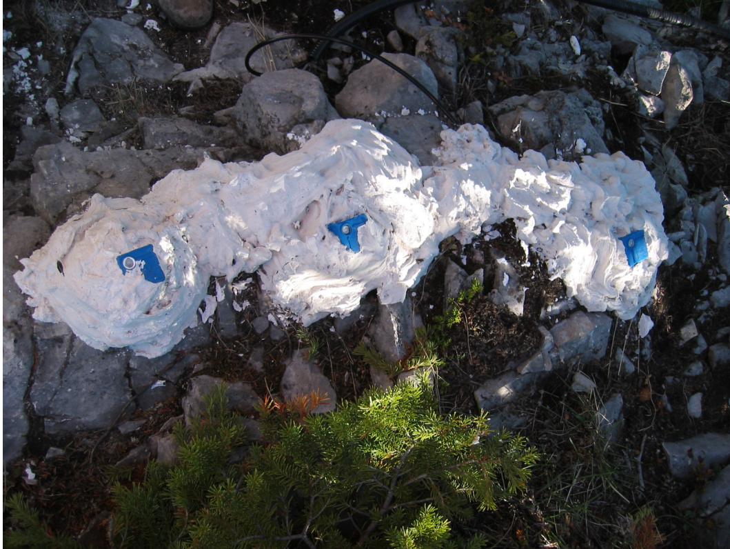
Figure 20. Geophones installed in outcrop on Turtle Mountain.
