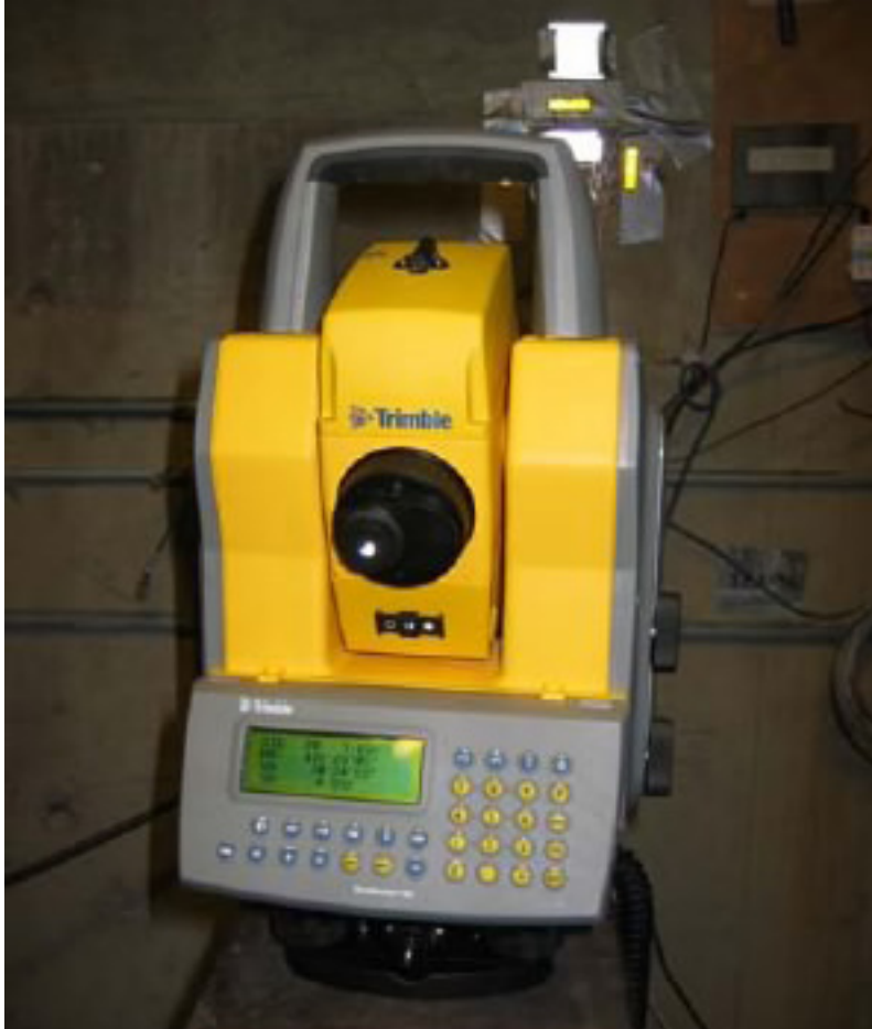
Figure 15. Trimble theodolite installed in the attic of the FSIC, viewing Turtle Mountain through a hole cut through the concrete wall of the building.
