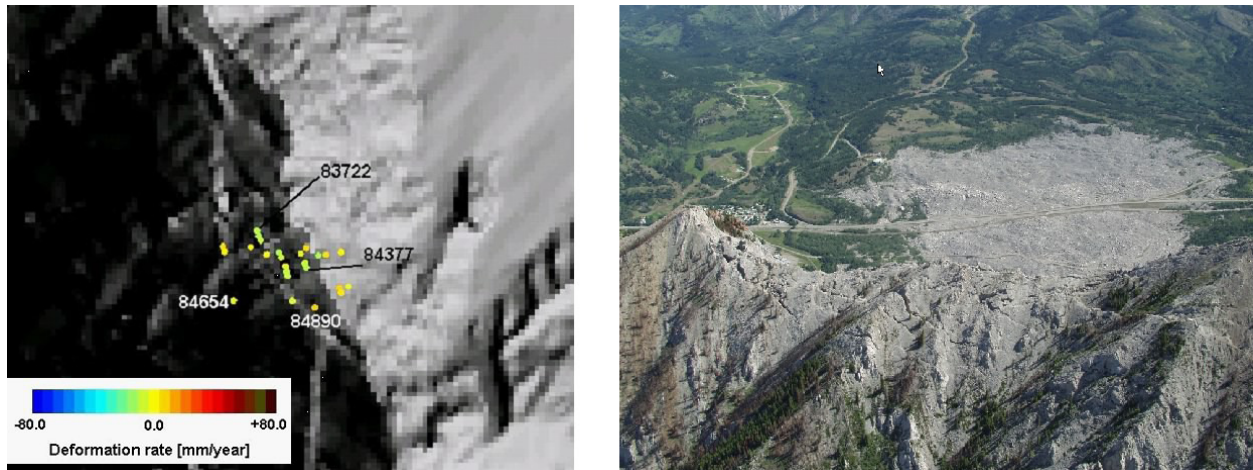
Figure 56. (left) Detected coherent target monitoring points for area 1 superimposed on digital elevation model ). (right) Oblique airphoto of the headscarp of the 1903 slide (area 1), showing the fractured and blocky terrain ( modified from Vexcel Canada, 2005 ).
