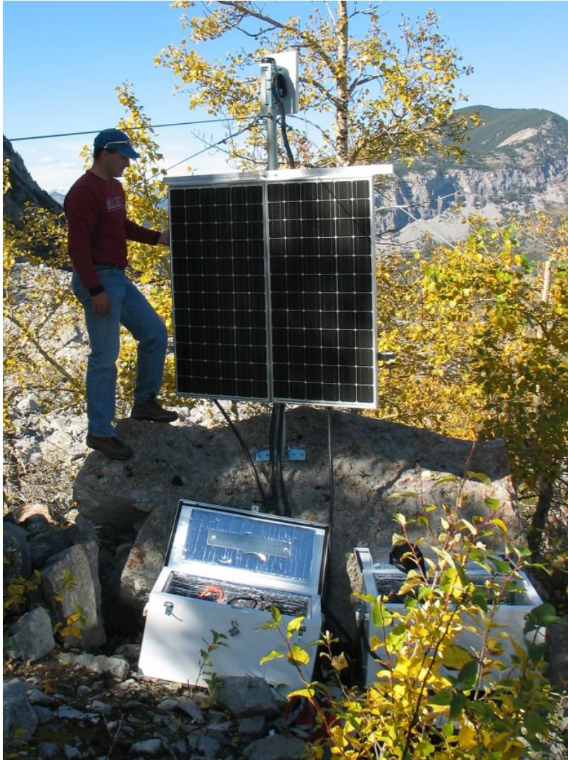
Figure 29. Solar power system on Turtle Mountain: Upgraded system at Pit station now provides double the generating and storage capacity.
