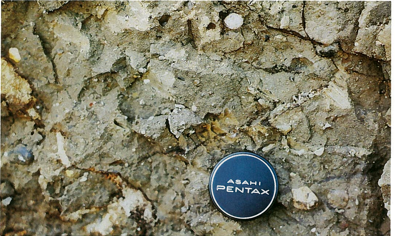
Plate 1b. Close-up view of freshly exposed oxidized till, Marie Creek Formation. Note iron staining along fracture planes. Section SRA-200 (LSD 11, Sec 1, Tp 63, R 3, W 4 Mer).
