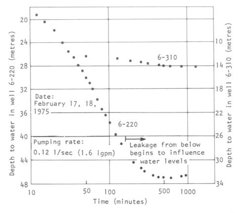
FIGURE 28. Water levels in wells 6-220 and 6-330 during pumping test on 6-220
