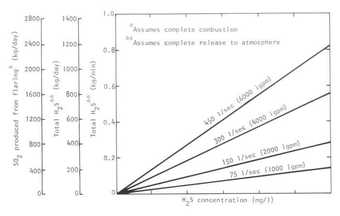
FIGURE 34. Hydrogen sulfide and sulfur dioxide production from pumping wells
