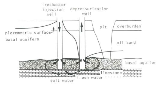
FIGURE 32. Pressure ridge method of salt water control
