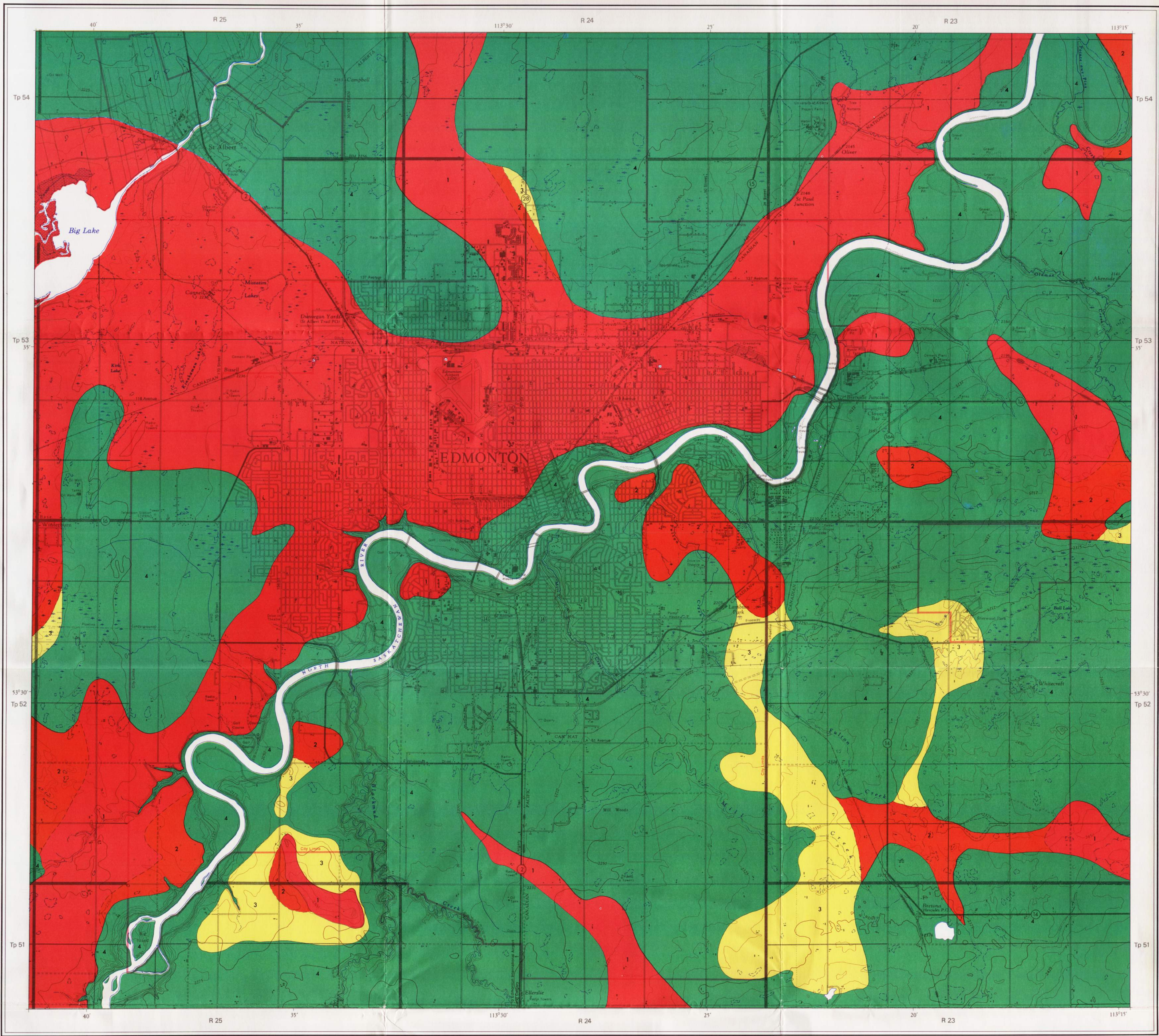
FIGURE 45. SUITABILITY OF THE EDMONTON AREA FOR DEEP SEWER CONSTRUCTION AT DEPTHS GREATER THAN 100 FEET (30 M) BELOW THE SURFACE.
