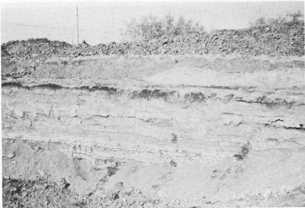
Figure 2. Rhythmically bedded glacial Lake Edmonton sediments consisting primarily of silt and clay (sewer excavation in west Edmonton near the junction of 170 St. and Quesnel Freeway).
